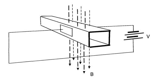
Two metal plates are placed on opposite sides of the tube, and a potential V is applied between them so that the charged particles in the liquid begin to flow across the tube At the same time, a magnetic field B is applied at right angles to the electric field produced by the plates
