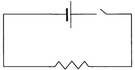
(a) Explain why a battery is essential in this circuit [4 marks] (b) In a particular torch, the light globe has a resistance of 20  $\Omega$  If the battery emf is 3 0 V, what is the current in the light globe? [4 marks] (c) Calculate the power at which the light globe operates, and hence how much energy the light globe uses when it operates for 10 minutes [6 marks] THIS PAGE HAS BEEN LEFT BLANK INTENTIONALLY
