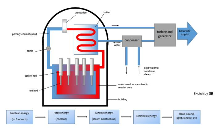
The energy from the coolant is then passed to pipes containing water. The water is converted into steam and this steam is used to rotate the turbines which drive generators. The generators produce electricity for use in industry or homes.
