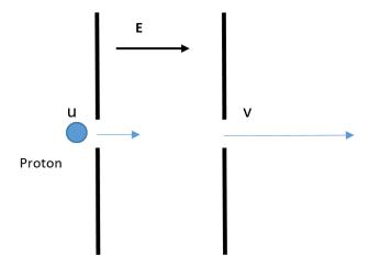
The electric field is now tripled (it becomes 3E). If another proton, having an initial kinetic energy KE<sub>initial</sub> enters the field, determine this proton's final kinetic energy in terms of KE<sub>initial</sub>. You should ignore the effects of gravity.
