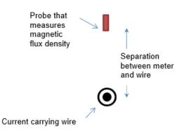
fed into the wire from an external power supply. The probe that measures magnetic flux density is placed at set distances from the middle of the wire and measurements recorded.
