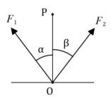
(a) Determine the magnitude of resultant force and the angle it makes with the vertical.
