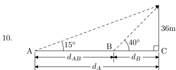
$$\begin{aligned}\tan 15^\circ &= \frac{36}{d_A} \\ d_A &= \frac{36}{\tan 15^\circ} \\ \tan 40^\circ &= \frac{36}{d_B} \\ d_B &= \frac{36}{\tan 40^\circ} \\ d_{AB} &= \frac{36}{\tan 15^\circ} - \frac{36}{\tan 40^\circ} \\ &= 91\text{m}\end{aligned}$$
