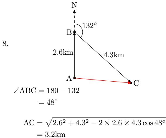
We'll initially find  $\angle BCA$  rather than  $\angle BAC$  because the sine rule is ambiguous for  $\angle BAC$  but  $\angle BCA$  can not be obtuse (because it is opposite a smaller side).
