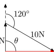
$$\begin{aligned} m &= \sqrt{5^2 + 10^2 - 2 \times 5 \times 10 \cos 60^\circ} \\ &= \sqrt{25 + 100 - 100 \times \frac{1}{2}} \\ &= \sqrt{75} \\ &= 5\sqrt{3} \\ \theta &= 090^\circ \end{aligned}$$
