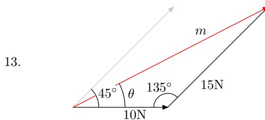
$$\begin{aligned}m &= \sqrt{10^2 + 15^2 - 2 \times 10 \times 15 \cos 135^\circ} \\ &= 23.2\text{N} \\ \frac{\sin \theta}{15} &= \frac{\sin 135^\circ}{23.2} \\ \theta &= \sin^{-1} \frac{15 \sin 135^\circ}{23.2} \\ &= 27^\circ\end{aligned}$$
