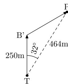
$$\begin{aligned} B'P &= \sqrt{250^2 + 464^2 - 2 \times 250 \times 464 \cos 32^\circ} \\ &= 286\text{m} \end{aligned}$$
