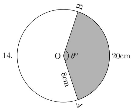
$$\begin{aligned}\theta &= l/r \\&= 20/8 \\&= 2.5 \\a &= \frac{1}{2}r^2\theta \\&= \frac{1}{2} \times 8^2 \times 2.5 \\&= 80\text{cm}^2\end{aligned}$$
