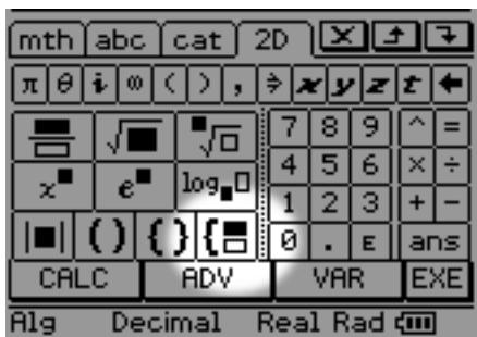
In the Main application, select the simultaneous equations icon in the 2D tab. Enter the two equations to the left of the vertical bar, and the two variables to the right:
