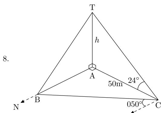
$$\begin{aligned}(a) \tan 24^\circ &= \frac{h}{50} \\ h &= 50 \tan 24^\circ \\ &\approx 22\text{m}\end{aligned}$$
