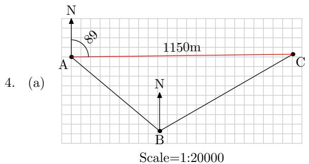
(b) Bearing of A from C is  $89 + 180 = 269^\circ$
