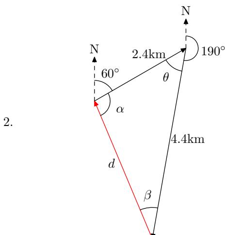
$$\begin{aligned} \theta &= 369 - 190 - (180 - 60) \\ &= 50^\circ \\ d &= \sqrt{2.4^2 + 4.4^2 - 2 \times 2.4 \times 4.4 \cos 50^\circ} \\ &= 3.4 \text{ km} \end{aligned}$$
