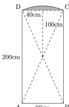
$$\begin{aligned} \text{Area} &= \frac{1}{2}r^2(\theta - \sin \theta) \\ &= \frac{1}{2} \times 107.7^2(0.761 - \sin 0.761) \\ &= 414\text{cm}^2 \end{aligned}$$
