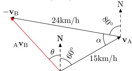
$$\begin{aligned}60 + (80 + \alpha) &= 180 \text{ (cointerior angles)} \\ \alpha &= 40^\circ\end{aligned}$$
