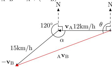
$$\begin{aligned}\alpha &= 360 - 90 - 120 \\ &= 150^\circ\end{aligned}$$
