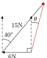
$$\begin{aligned} m &= \sqrt{6^2 + 15^2 - 2 \times 6 \times 15 \cos 50^\circ} \\ &= 12.1 \text{ N} \\ \frac{\sin(\phi)}{6} &= \frac{\sin 50}{12.1} \\ \phi &= \sin^{-1} \frac{6 \sin 50}{12.1} \\ &= 22^\circ \\ \theta &= 180 - 90 - 50 - 22^\circ \\ &= 018^\circ \end{aligned}$$
