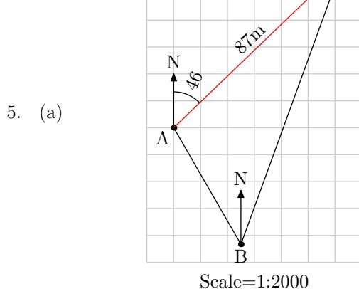
(b) Bearing of A from C is  $46 + 180 = 226^\circ$
