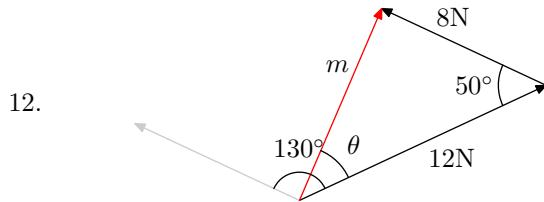
$$\begin{aligned}m &= \sqrt{8^2 + 12^2 - 2 \times 8 \times 12 \cos 50^\circ} \\ &= 9.2\text{N} \\ \frac{\sin \theta}{8} &= \frac{\sin 50^\circ}{9.2} \\ \theta &= \sin^{-1} \frac{8 \sin 50^\circ}{9.2} \\ &= 42^\circ\end{aligned}$$
