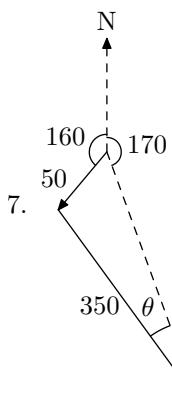
$$\begin{aligned}\frac{\sin \theta}{50} &= \frac{\sin 30^\circ}{350} \\ \theta &= \sin^{-1} \frac{50 \sin 30^\circ}{350} \\ &\approx 4.1^\circ\end{aligned}$$
