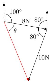
$$\begin{aligned} m &= \sqrt{8^2 + 10^2 - 2 \times 8 \times 10 \cos 80^\circ} \\ &= 11.7 \text{ N} \\ \frac{\sin \theta}{10} &= \frac{\sin 80}{11.7} \\ \theta &= \sin^{-1} \frac{10 \sin 80}{11.7} \\ &= 58^\circ \\ \text{bearing} &= 100 + 58^\circ \\ &= 158^\circ \end{aligned}$$
