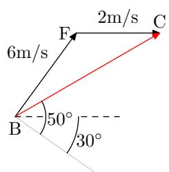
$$\begin{aligned}\angle C &= 50 - 30 \\ &= 20^\circ \\ \frac{\sin \angle B}{2} &= \frac{\sin 20^\circ}{6} \\ \angle B &= \sin^{-1} \frac{2 \sin 20^\circ}{6} \\ &= 6.5^\circ\end{aligned}$$
