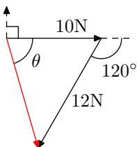
$$\begin{aligned} m &= \sqrt{12^2 + 10^2 - 2 \times 12 \times 10 \cos 60^\circ} \\ &= \sqrt{144 + 100 - 240 \times \frac{1}{2}} \\ &= \sqrt{124} \\ &= 2\sqrt{31} \\ \sin \theta &= \frac{\sin 60}{2\sqrt{31}} \\ \theta &= \sin^{-1} \frac{12 \sin 60}{2\sqrt{31}} \\ &= 69^\circ \end{aligned}$$
