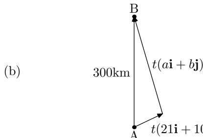
We must add the helicopter's own velocity to the wind velocity to produce a resultant headed due North.
