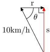
The speed of the boat's movement across the river ( $s$ ) can be determined using Pythagoras:
