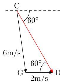
$$\begin{aligned}\frac{\sin \angle C}{2} &= \frac{\sin 60^\circ}{6} \\ \angle C &= \sin^{-1} \frac{2 \sin 60^\circ}{6} \\ &= 16.8^\circ\end{aligned}$$
