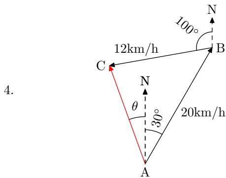
$$\begin{aligned}\angle ABC &= 180 - 30 - 100 \\&= 50^\circ \\AC &= \sqrt{20^2 + 12^2 - 2 \times 20 \times 12 \cos 50^\circ} \\&= 15.3 \text{ km/h}\end{aligned}$$
