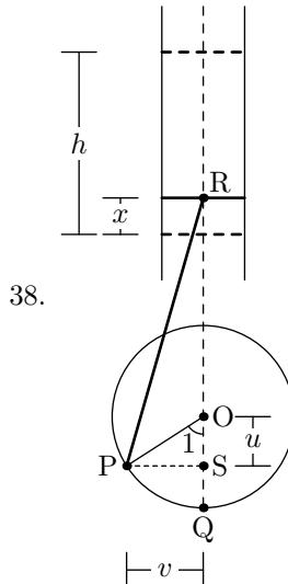
The lowest position of the piston is  $r$  above the top of the wheel. Therefore it is  $3r$  above the bottom of the wheel. Thus the fixed length of the drive rod  $PR = 3r$ .
