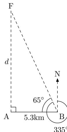
$$\begin{aligned}\angle ABF &= 335 - 270 \\ &= 65^\circ\end{aligned}$$
