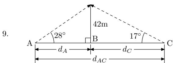
$$\begin{aligned}\tan 28^\circ &= \frac{42}{d_A} \\ d_A &= \frac{42}{\tan 28^\circ} \\ \tan 17^\circ &= \frac{42}{d_C} \\ d_C &= \frac{42}{\tan 17^\circ} \\ d_{AC} &= \frac{42}{\tan 28^\circ} + \frac{42}{\tan 17^\circ} \\ &= 216\text{m}\end{aligned}$$
